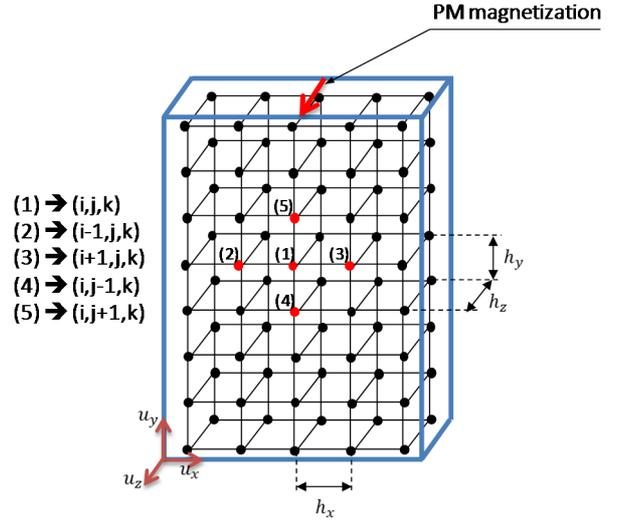
Fig. 1. PM mesh grid used for 3-D FDM.
