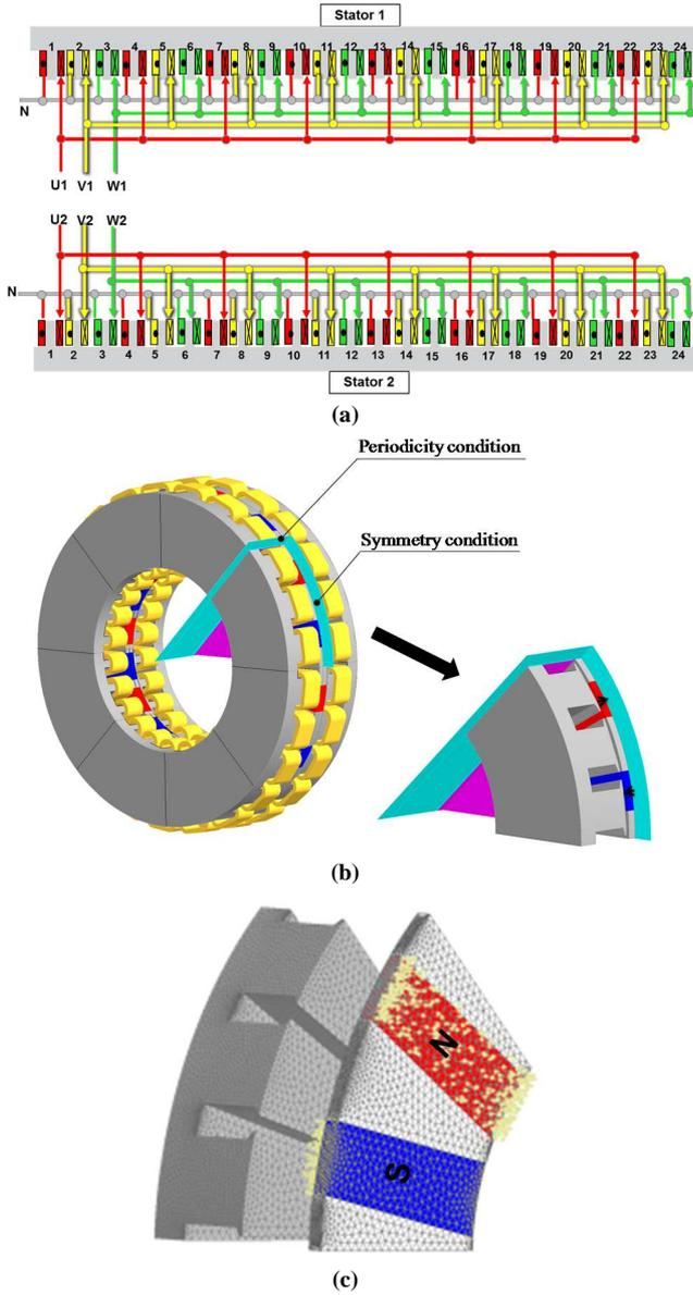
Fig. 2. Axial-flux PMSM (24-slots/16-poles) studied: (a) non-overlapping winding, (b) reduced SPM machine, and (c) mesh.
