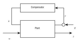
Figure 1 - Block diagram of a typical feedback control setup, including plant, compensator, external noise sources (w, g) and objective output z
