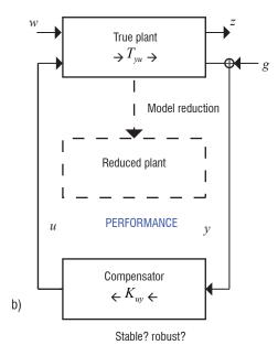
Figure 6 - a) Design of a compensator based on a reduced-order model of the true plant. b) Application of the designed compensator to the full model of the true plant
