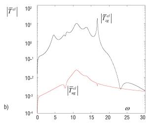
Figure 3 - a) Open-loop transfer function  $|T_{yu}(\omega)|$  of the full plant (black dashed line) and of reduced- order models based on the four unstable global modes and no (blue), four (green) and eight (red) balanced POD modes to represent the stable subspace. b) Closed-loop transfer functions from the measurement noise g to the sensor output z (black) and from the measurement noise g to the control input u (red).
