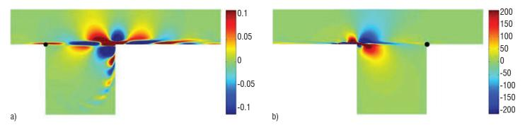
Figure 4 - Dominant balanced modes computed by the bPOD method for flow over an open cavity (visualized by streamwise velocity contours). a) The dominant direct mode, determined from the impulse responses of the actuator location (black symbol); b) the adjoint mode, determined from the adjoint impulse response of the sensor location (black symbol).
