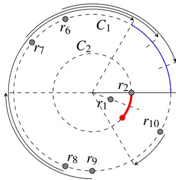
(d) Execution of *removeRobotsInExcess(i)* when  $i = 1$ : the 3 greatest robots form the regular 3-gon, and the other robots are evenly distributed on blue arc.
