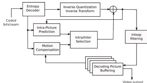
**Fig. 1.** Simplified diagram of an HEVC decoder.
