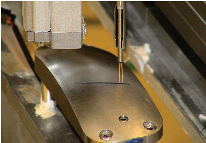
Figure 27 - Hot-wire qualification of an actuator as a wind tunnel model component
