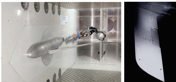
Figure 1 - DTP Modèles 3 – half-model in the S2MA wind tunnel (left) and detailed view of the R/C aileron (right)
