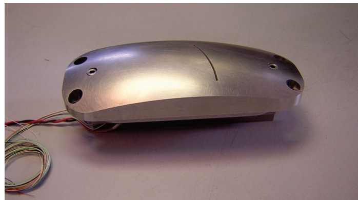
Figure 21 - One synthetic jet before integration into the model
