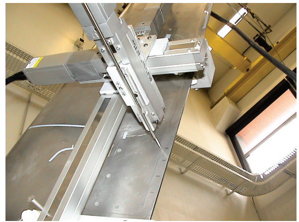
Figure 33 - In-situ hot-wire probing of a fluidic trailing edge device (TED). The probe is mounted on a high accuracy, motorized robot with 3 degrees of freedom
