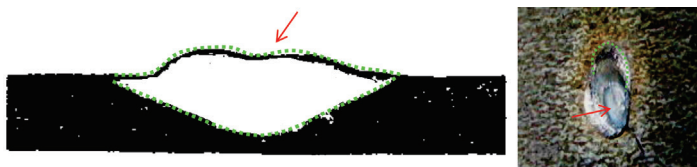
Figure 18 - Picture on the left, section through the center of the cathode spot (Dobbing & Hanson, 1978). Picture on the right, view of a cathode spot for an 800A, 200C arc on an aluminum panel (DGA-TA). The drop of metal is deformed by gravity.
