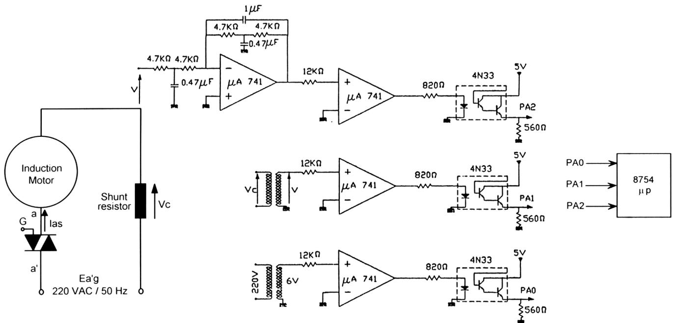
(PA0: Mains voltage, PA1: motor voltage, PA2: Motor current fundamental component)
