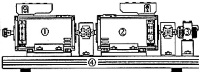
(1. DC motor, 2. DC generator, 3. Impulse transmitter, 4. Base)
