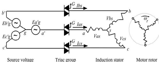
Fig. 3. Induction motor voltage controller.
