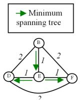
Figure 4. Minimum spanning tree covering all the nodes of the transitive graph
