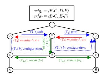
Figure 3. Message sequencing for the setup of a primary protected LSP ( $A \rightarrow B \rightarrow C$ )
