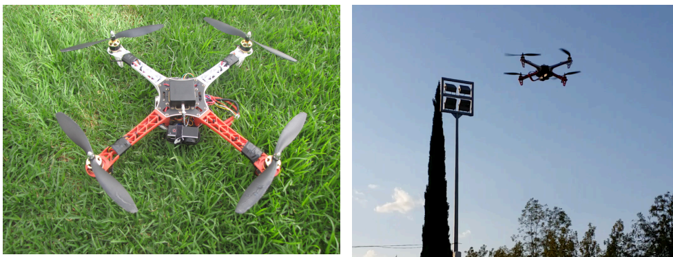
Figure 4. The quadrotor mini-helicopter in flight.
