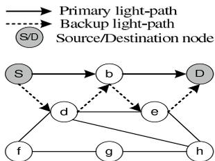
Fig. 1 Link-based protection
