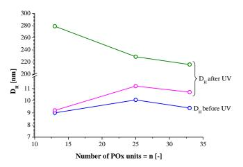
**Fig 6.** Hydrodynamic diameter ( $D_H$ ) determined using DLS as a function of the length of the POx block for CoumC<sub>11</sub>-POx<sub>n</sub> before and after UV-irradiation (direct dissolution in water at 4 mg mL<sup>-1</sup>).
