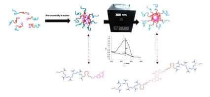
**Scheme 3.** Principle of the photo-dimerization of self-organized CoumC<sub>11</sub>-POx<sub>n</sub>.
