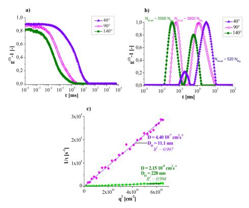
**Fig 5.** DLS results of CoumC<sub>11</sub>-POx<sub>25</sub> directly dissolved at 4 mg mL in water after UV-irradiation. (a, b) autocorrelation function ( $g^{(2)}$ -1) as a function of time (t) and relaxation time distribution at scattering angles of 40, 90 and 140°, and (c) dependence of  $\Gamma$  on  $q^2$  from 15 up to 150° by step of 5° (coefficient of determination for the linear regression ( $\mathbb{R}^2$ )).
