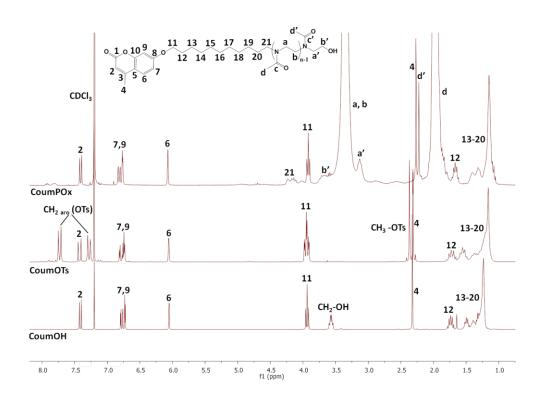
Fig 1. <sup>1</sup>H NMR spectra (300 MHz; CDCl<sub>3</sub>) of CoumOH, Coum-OTs and CoumC<sub>11</sub>-POx<sub>n</sub>.
