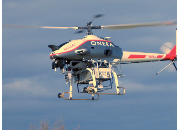
Figure 3 - An Onera ReSSAC unmanned helicopter
