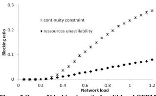
Figure 5 Cause of blocking in optical multi-band OFDM network
