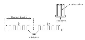
Figure 1 Typical Optical Multi-band OFDM Spectrum
