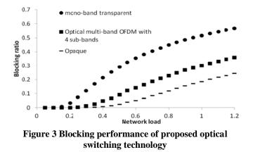
As expected, the blocking ratio is higher in mono-band transparent network than in optical multi-band OFDM network and mono-band opaque network. This is due to the fact that in mono-band transparent switching, each requests uses an entire optical channel, while in the case of optical multi-band OFDM switching and the mono-band opaque switching an optical channel can be shared by multiple requests.
