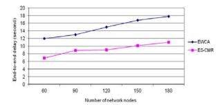
Fig. 4. End-to-end delay versus number of nodes
