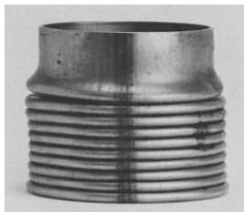
(a) Crushed circular tube test specimens [ABR86]
