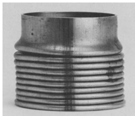
(a) Crushed circular tube test specimens [ABR86]
