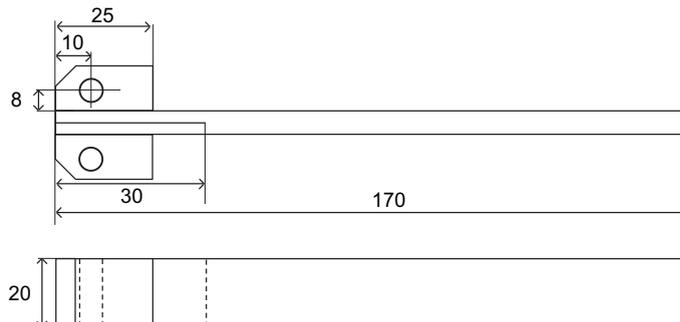
Fig. 1. Dimensions of DCB specimens and experimental set-up.
