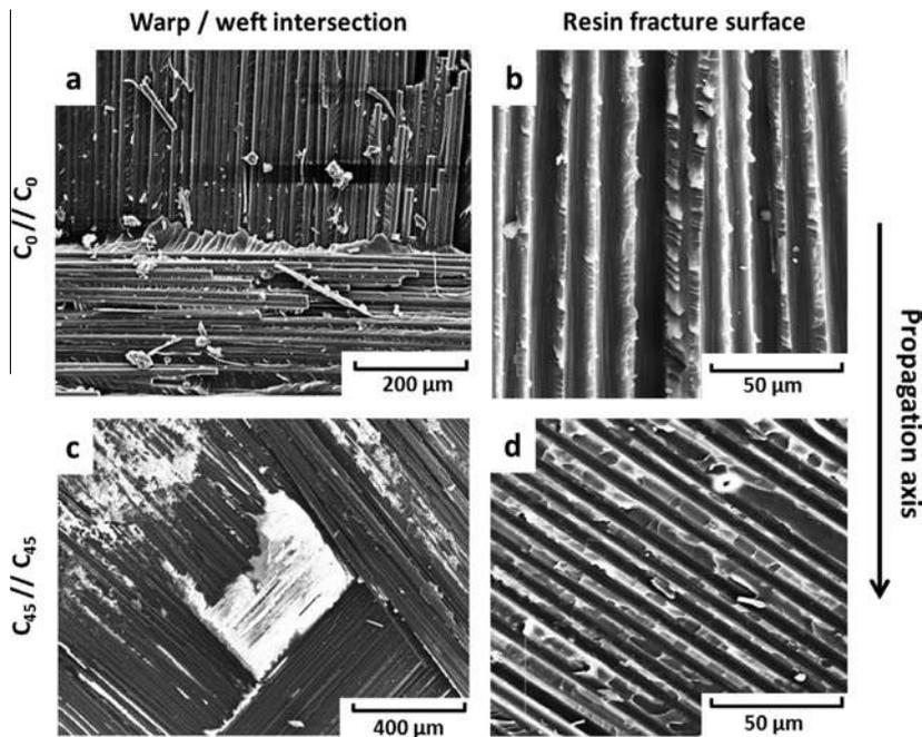
Fig. 6. Scanning electron microscope view of the fracture surfaces for different woven fabric ply orientation.
