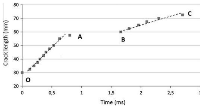
Fig. 3. Two regimes of the crack propagation.
