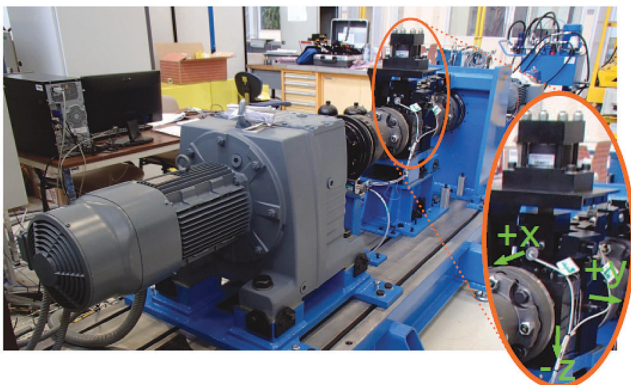
Figure 2. The test-rig. The main bearing is marked by an orange ellipsis and the three accelerometer directions are symbolised by the green arrows
