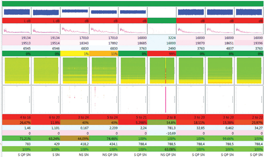
Figure 2. The behaviour of AStrion-D over time. The green colour is OK and the red colour is ALARM. S is for stationary, QP is for quasi-periodic and SN is for significant noise
