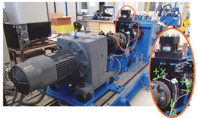
Figure 1. The wind turbine test-bench. The orange ellipsis circles zoom into the main bearing and its loading unit, while the green arrows represent the three wired accelerometers
