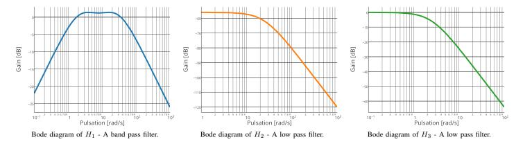
Fig. 5: Bode diagrams of the three designed filters  $H_1$ ,  $H_2$  and  $H_3$ , with  $f_1 = 4$  Hz and  $f_2 = 0.4$  Hz.
