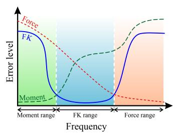
Fig. 3: A sketch representation of the spectral distribution of errors that would emerge from the naive reconstruction of CoM trajectory if we use only one signal (Geometry, Forces and projection of the CoM from Geometry onto the Contact Wrench Central Axis). The signal with the lowest error is then selected at each frequency bandwidth to constitute minimal-error fusion of these signals.
