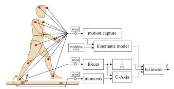
Fig. 1: The problem of merging measurements for CoM reconstruction in the presence of noises and modeling errors.
