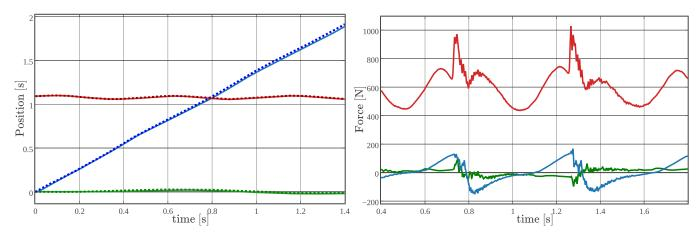
Fig. 8: CoM position reconstruction for natural walking (blue for x, green for y and red for z). On the left, the reconstructed CoM in plain line and the CoM coming from geometry in dotted line. On the right the force measurement.
