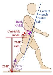
Fig. 2: A graphic representation of the comparison between the central axis of the contact wrench and the ZMP. The ZMP part is depicted in red and shows the approximation made by the cart table model. The line joining the ZMP to the CoM of the cart-table model is parallel to the contact force vector. The central axis part is shown in blue. It is the line of minimal moment norm, also parallel to the contact force vector.
