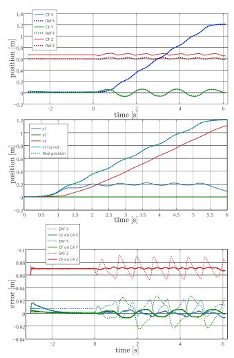
Fig. 7: On the top, the reconstructed trajectory thanks to the complementary filter. On the middle, the plot shows the contribution of every signal to the reconstruction of CoM trajectory along  $\boldsymbol{x}$  axis together with the sum of the signals. The dotted line represents the ground truth value. On the bottom, error between the ground truth measure of the CoM position and its reconstruction with the Kalman filter and the complementary filter.
