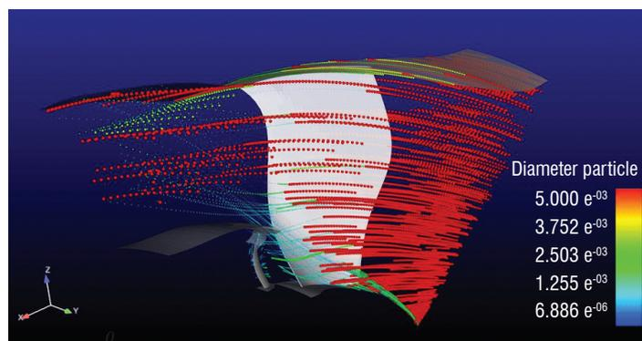
Figure 2 – Example of hail particle trajectories colored by their diameter through a turbojet engine (fan and IGV)
