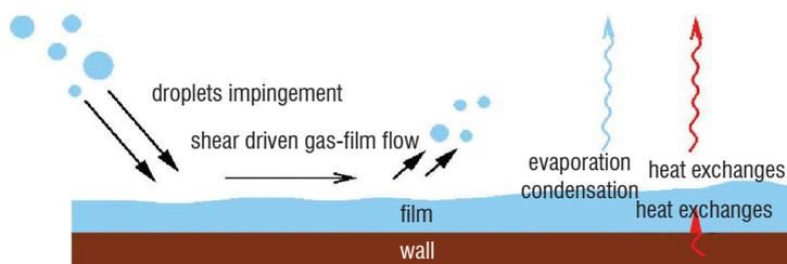
Figure 3 – Wall liquid films formed under multi-physics configurations
