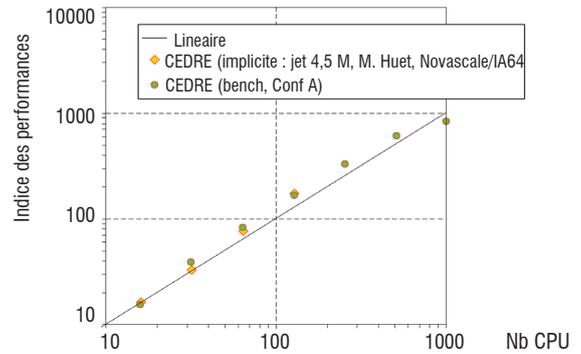
Figure 5 – Example of CEDRE performance on parallel computers
