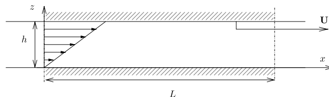
FIG. 15. Plane Couette flow: the time of flight is calculated with Poincaré sections being separated by a length L .
