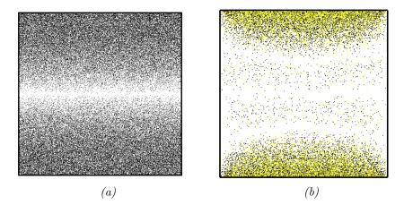
FIG. 2. Poincaré sections (plane (x = 0.5)) for: (a) the slipping wall cavity flow in the case of global chaos  $U_1 = 0.25$ ; (b) the no-slip walls cavity flow: in this case, two Poincaré sections are superimposed, represented by two different colors in the online version.
