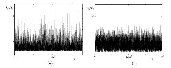
FIG. 7. Non-dimensional time of flight,  $t_f/\bar{t}_f$ , versus the ordinal number of Poincaré section points, n for a unique trajectory, corresponding to: (a) one of the Poincaré sections in figure 6.a (multi-level laminating mixer); (b) the trajectory in figure 2.a (slipping-walls cavity flow).
