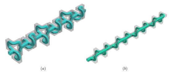
FIG. 5. Geometry and iso-surface of velocity modulus plot for a Stokes flow inside: (a) the Multi-level laminating mixer (6 elements); (b) the "F" mixer of Chen and Meiners<sup>44</sup> (8 elements).
