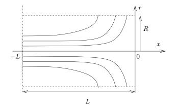
FIG. 11. Flow in the vicinity of an hyperbolic point (located here at (x = r = 0)). We define a domain  $\mathcal{D} = (-L \leq x \leq 0) \times (r \leq R)$  around this fixed point; the waiting time in  $\mathcal{D}$ , denoted by  $\tau$ , is the time it takes to move from the plane (x = -L) up to the cylinder (r = R).
