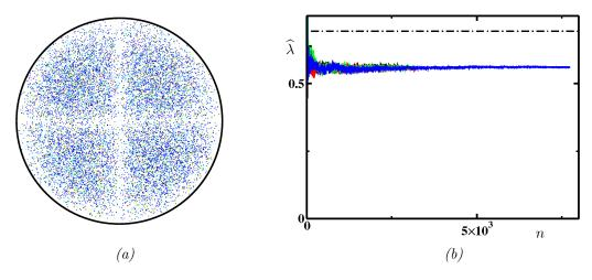
FIG. 4. Kenics mixer: (a) Poincaré sections (four sections are superimposed); (b) convergence of the positive Lyapunov exponent with the number of mixing elements n; the dot-dashed line is  $\ln(2)$ .
