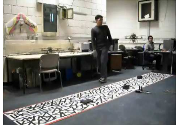
Fig. 1. Position stabilization and velocity regulation of a quad-rotorcraft during an autonomous flight. The proposed strategy makes use of a monocular imaging system and is based on optical flow computation.
