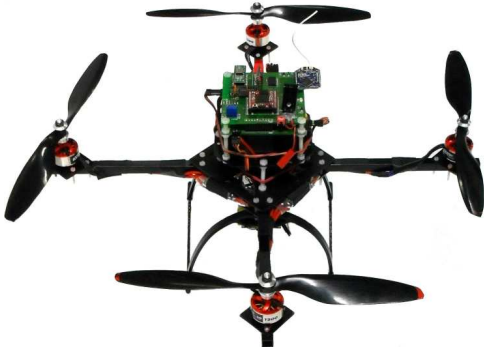
Fig. 4. Four rotor helicopter equipped with a camera.
