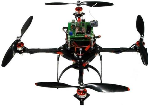
Fig. 4. Four rotor helicopter equipped with a camera.
