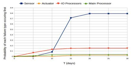
Figure 7: The probability that each of the 4 failure types is the cause of system shutdown in the first T time of operation
