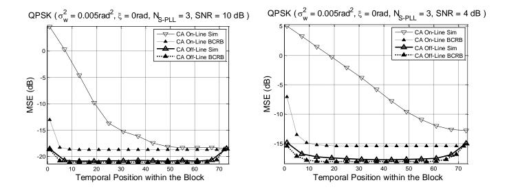
Fig. 3 MSE curves for the various positions in the block at two different SNRs.
