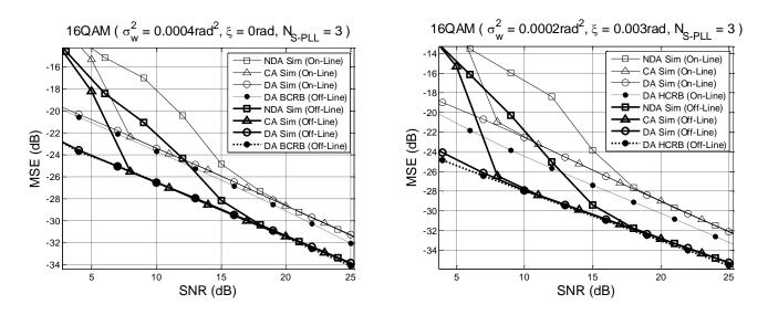
Fig. 6 16QAM performance in the center position versus SNR for two different linear drifts
