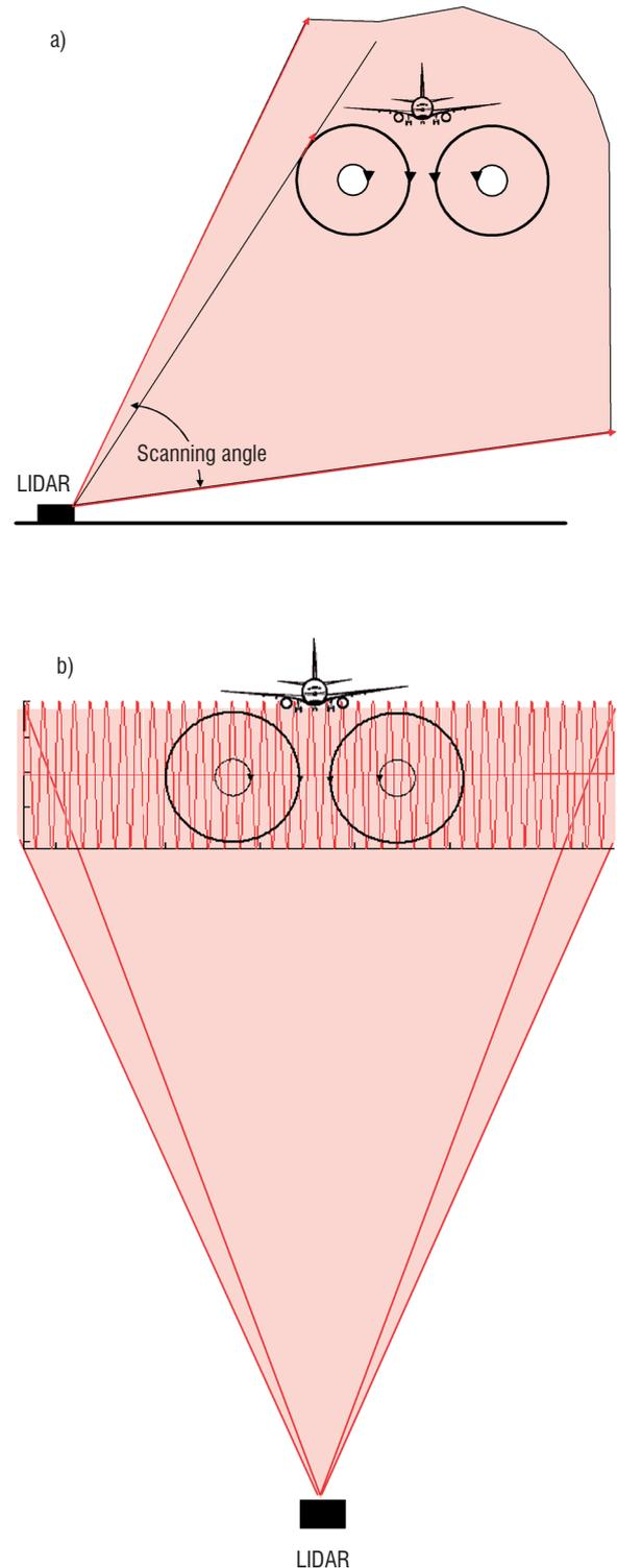
Figure 2 - Lidar scanning pattern: (a) for lateral wake vortex detection, (b) for axial wake vortex detection.
