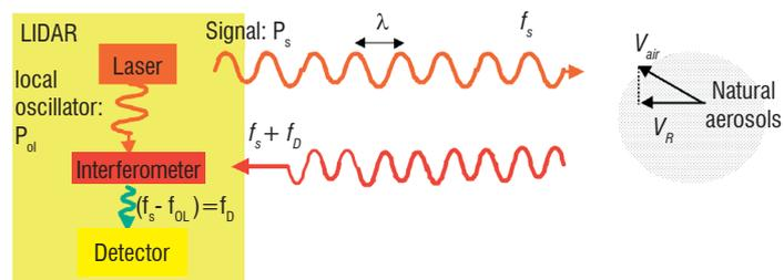
Figure 1 - Coherent detection lidar principle.
