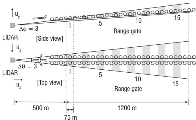
Figure 17 - Scanning configuration.
