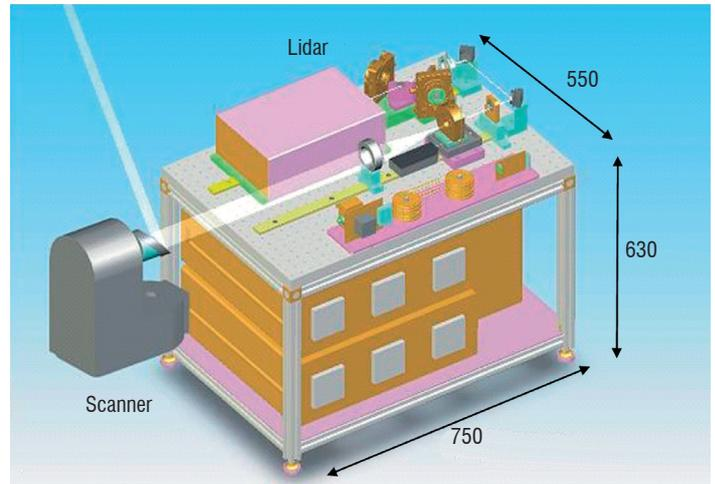
Figure 9 - Drawing and size of SWAN lidar.
