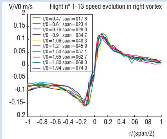
Figure B2-03 - Field test wake vortex measurements with Onera CW lidar: normalized velocity profile evolution.
