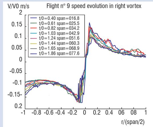
Figure B2-04 - Catapult (reduced-scale) vortex measurements with CW mini-lidar: normalized velocity profile evolution.
