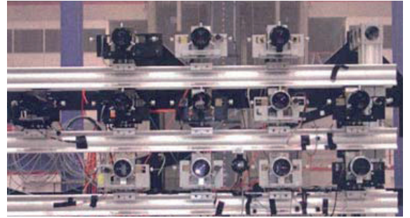
12 PIV cameras mounted on rails
