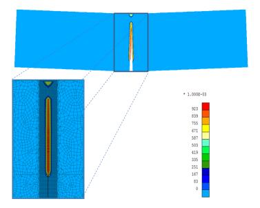
FIGURE 1 - 3 point bending test : Damage distribution at the notch tip with open cohesive zones
