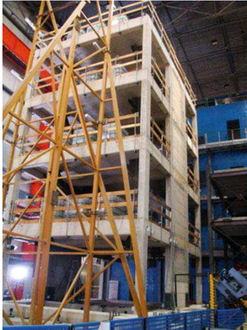
Fig. 3 Elevation of the specimen in the lab. The wall shown on the right is the South wall (frame) and the one on the left is the North wall (frame)
