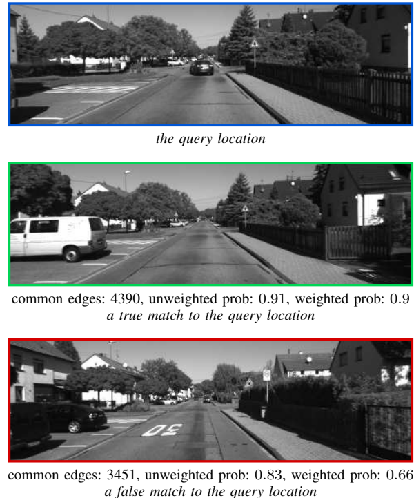
Fig. 6: Example of a query and two retrieved locations from the KITTI dataset. In this case, both of the retrieved location graphs share many common edges with the query. As a result, the match probabilities when using unweighted term frequencies are high for both locations. However, when using term frequencies, which are weighted by the relative document frequencies from sample locations, the match probability of the false candidate drops significantly.
