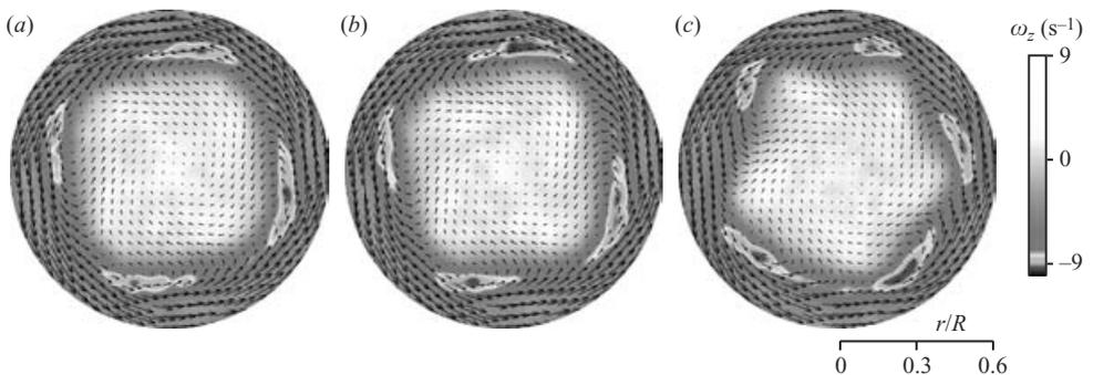
FIGURE 15. Experimental velocity and vorticity fields for  $\Gamma = 3$  and  $Re_t = 280$ . (a)  $Re_b = 75$ ; (b)  $Re_b = 77$ ; (c)  $Re_b = 79$ . The grey scale has been chosen in order to emphasize the local vorticity extrema of the shear layer.
