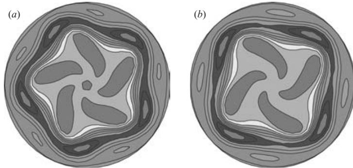
FIGURE 18. Iso-vorticity levels at mid-height obtained for the same parameters,  $\Gamma = 3$ ,  $Re_t = 280$ ,  $Re_b = 80$ , starting from different initial conditions: (a) from sudden increase of  $Re_b$  from 70, showing a mode  $m = 5$ ; (b) from progressive increase of  $Re_b$  from 70, showing a mode  $m = 4$ . Only the central circle  $r \leq 0.65R$  is shown.
