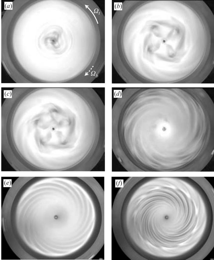
FIGURE 6. Instability patterns visualized by seeding flakes. (a)  $(\Gamma, Re_t, Re_b) = (6.1, 584, 79)$ , showing a mode  $m = 3$ . (b)  $(7, 282, 47.1)$ ,  $m = 4$ . (c)  $(7, 282, 51.8)$ ,  $m = 5$ . (d)  $(10.8, 60.6, 26.8)$ ,  $m = 7$ . (e)  $(20.9, 46, 10.5)$ ,  $m = 11$ . (f)  $(20.9, 74, 13.6)$ ,  $m = 11$ . The flow is only visible on a central region,  $r \leq 0.83R$ , due to the shadow from the cylindrical rim. Disk rotations are indicated by the arrows in (a).
