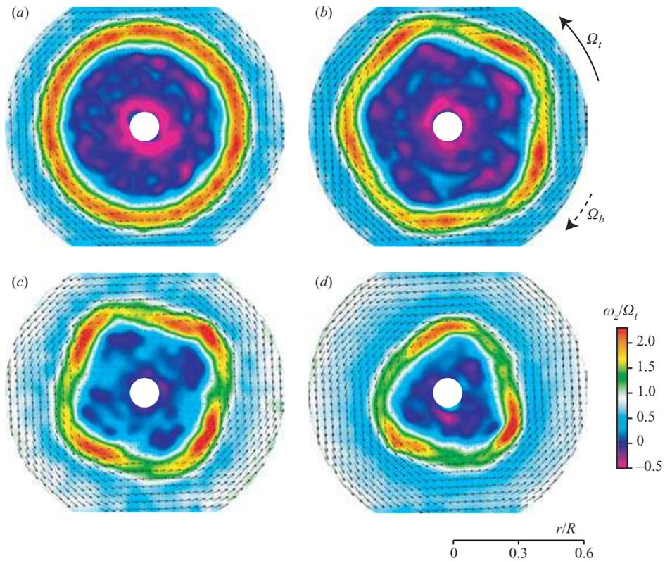
FIGURE 10. Experimental velocity and vorticity fields  $\omega_z$  at mid-height  $\Gamma = 7$ ; (a) is below the onset, and (b–d) are for increasing Reynolds numbers along the onset curve. (a)  $(Re_t, Re_b) = (240, 40)$ ; (b)  $(240, 43)$ ; (c)  $(289, 45)$ ; (d)  $(341, 50)$ .
