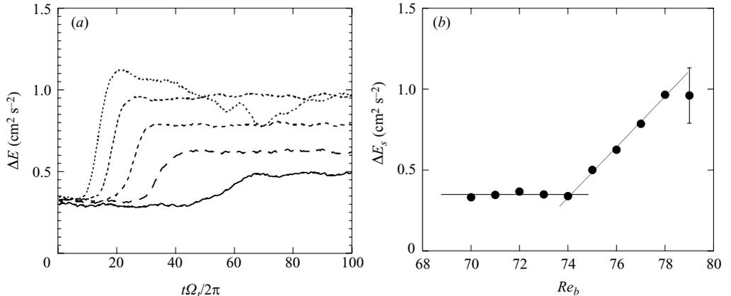
FIGURE 14. (a) Energy of the non-axisymmetric part of the flow, equation (5.1), as function of time, after a sudden increase of  $Re_b$  at  $t = 0$  s from 70 to 75, 76, 77, 78 and 79 (from solid line to short-dashed line), computed from the velocity fields of figure 15 ( $\Gamma = 3$  and  $Re_t = 280$ ). (b) Energy of saturation of the bifurcated state as a function of  $Re_b$ .
