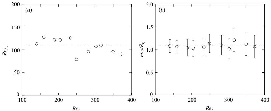
FIGURE 20. (a) Critical local Reynolds number  $Re_{l,c}$  based on the shear layer thickness as a function of  $Re_t$  for  $\Gamma = 7$ . For each measurement, the bottom Reynolds number  $Re_b$  is fixed to its transition value. (b) Corresponding normalized wavenumber  $m w / R_0$ .
