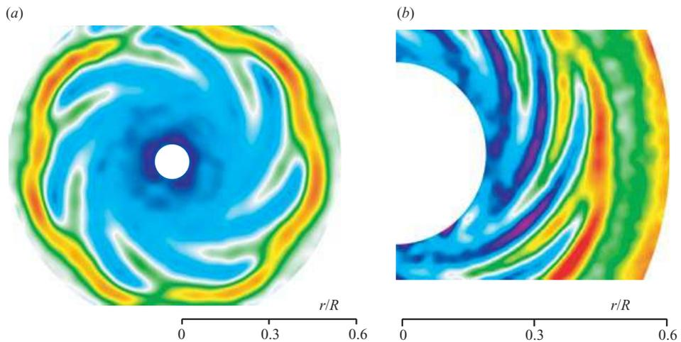
FIGURE 11. Experimental vorticity fields  $\omega_z$  at mid-height. (a)  $(\Gamma, Re_t, Re_b) = (9.3, 183, 28.5)$ , mode  $m = 7$ . (b)  $(14, 80, 19)$ , mode  $m = 8$ . The colour maps are the same as in figure 10.
