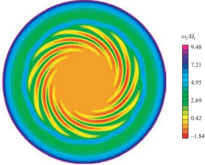
FIGURE 12. Numerical axial vorticity field  $\omega_z$  at mid-height  $z = h/2$  for  $\Gamma = 21$ ,  $Re_t = 67$ ,  $Re_b = 14.3$ , showing a mode  $m = 11$ . Only the central region  $r \leq 0.95R$  is shown.
