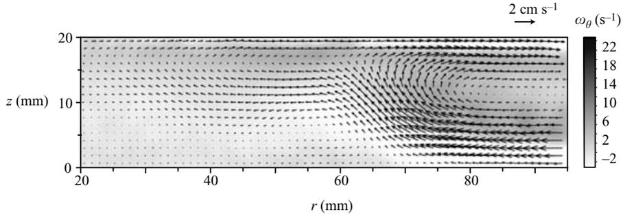
FIGURE 2. Experimental velocity field of the base flow in the meridional plane, and azimuthal vorticity field  $\omega_\theta$  (grey scale), for  $\Gamma = 7$ ,  $Re_t = 130$  and  $s = 0.154$ . Note that only the region  $0.14 \leq r/R \leq 0.68$  is shown.
