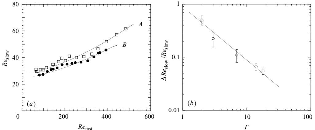
FIGURE 9. (a) Stability curves for an aspect ratio  $\Gamma = 7.2$ .  $\square$ , Configuration A: the sidewall rotates with the faster disk;  $\bullet$ , Configuration B: the sidewall rotates with the slower disk. (b) Relative deviation of the threshold between configurations A and B as a function of  $\Gamma$ . The line shows  $0.9\Gamma^{-1}$ , and the error bars reflect the variability of the deviation along the curves from (a).
