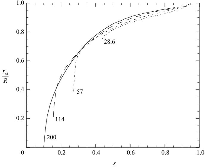
FIGURE 4. Normalized stagnation radius  $r_{st}/R$  as a function of the counter-rotation ratio  $s = Re_b/Re_t$  for  $\Gamma = 7$ , from axisymmetric simulations. The corresponding Reynolds number of the top disk,  $Re_t$ , is indicated.
