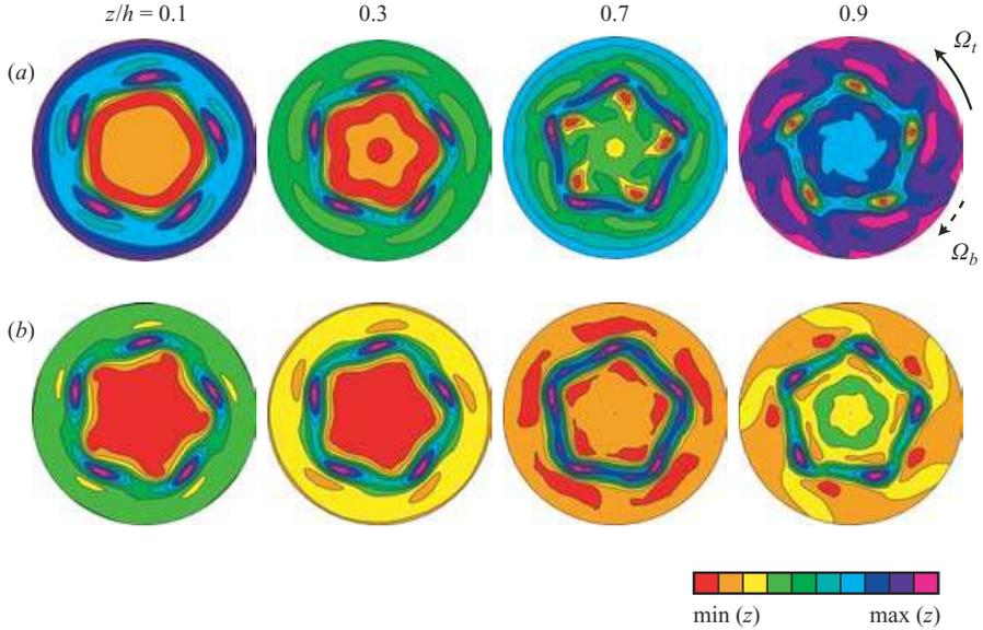
FIGURE 13. Numerical axial vorticity  $\omega_z$  (a) and axial velocity  $v_z$  (b) at different heights  $z/h = 0.1$  (close to the slower disk), 0.3, 0.7 and 0.9 (close to the faster disk), for  $\Gamma = 7$ ,  $Re_t = 250$ ,  $Re_b = 57$ , showing a mode  $m = 5$ . The colour maps for both  $\omega_z$  and  $v_z$  are normalized by their minimum and maximum on each field. Only the central region  $r/R \leq 0.6$  is shown.
