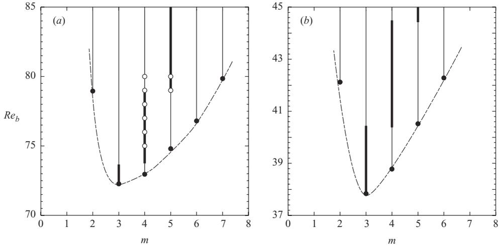
FIGURE 17. Marginal stability curves obtained from the linear computations for  $Re_t = 280$ . ●, critical Reynolds number  $Re_b$  for a given mode  $m$ ; thick line, most unstable mode. The dashed curve joining the points is guide for the eye. (a)  $\Gamma = 3$ ,  $Re_{b,c} = 72.3$ ; ○, experimentally observed modes. (b)  $\Gamma = 7$ ,  $Re_{b,c} = 37.8$ .
