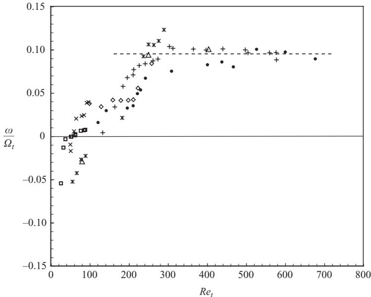
FIGURE 22. Normalized phase velocity  $\omega/\Omega_t$  at the onset as a function of  $Re_t$  for various aspect ratios  $\Gamma$ . Experiment:  $\diamond$ ,  $\Gamma = 3$ ;  $\bullet$ , 5.2;  $+$ , 7;  $\star$ , 9.3;  $\times$ , 17;  $\square$ , 20.9. Numerics:  $\triangle$ ,  $\Gamma = 7$ . The dashed line is  $\omega/\Omega_t = 0.095$ .
