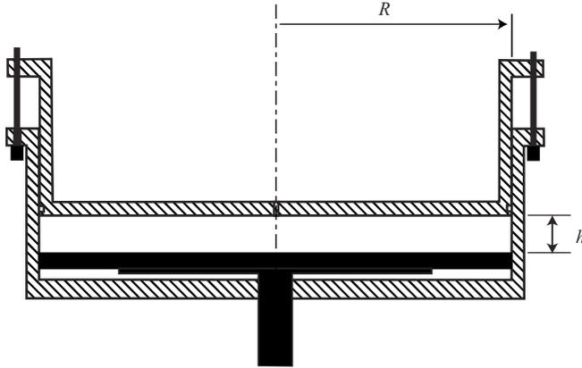
FIGURE 1. Experimental cell. The cylinder (hatched regions), made of transparent Plexiglas, rotates with angular velocity  $\Omega_t$ , while the bottom disk (black) rotates in the opposite sense with angular velocity  $\Omega_b$ .
