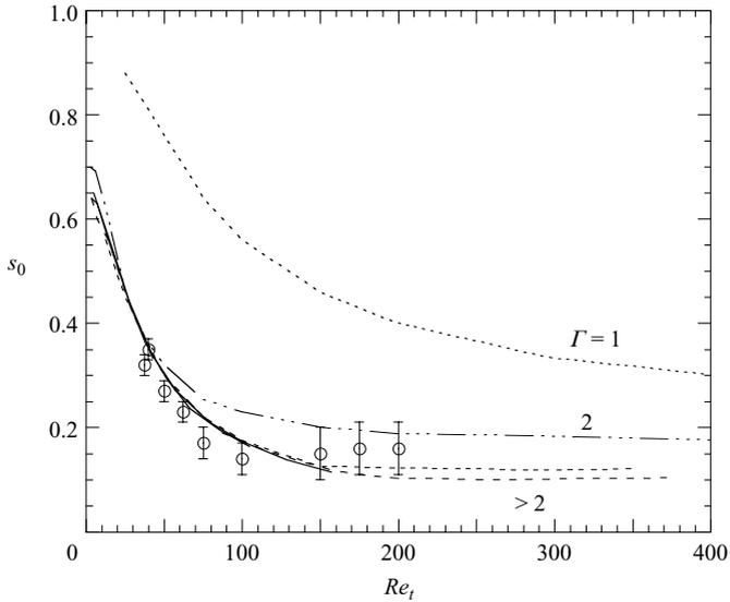
FIGURE 5. Critical counter-rotation ratio  $s_0$  as a function of  $Re_t$ . Lines: numerical results, for various aspect ratios,  $\Gamma = 1, 2, 4, 7, 14, 21$  and  $28$  (from top to bottom).  $\circ$ , Experimental measurements, for  $\Gamma = 20.9$ .
