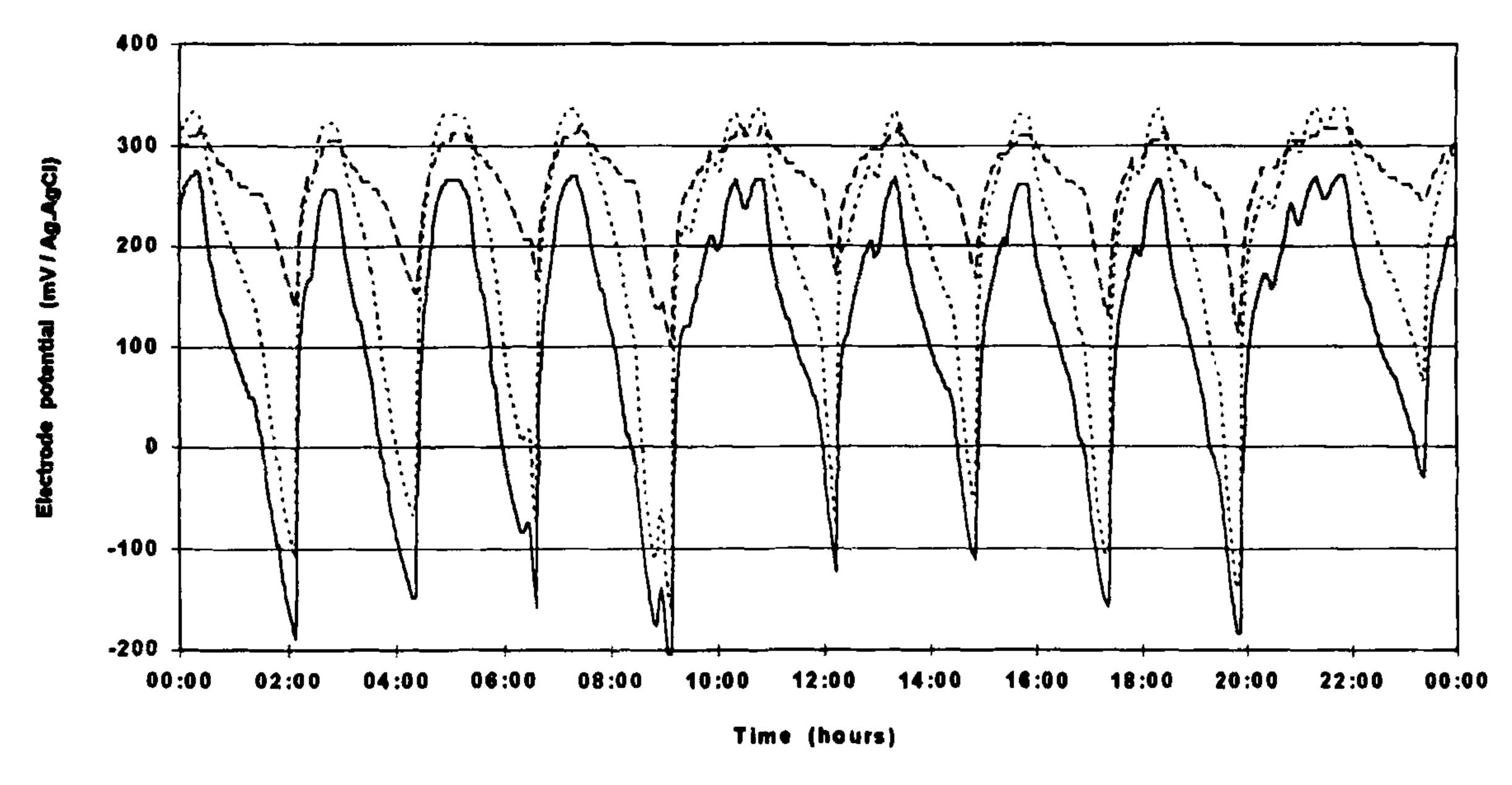
Figure 5. Comparative evolution of the potentials taken by (-) polished electrodes and electrodes coated with (...) a Nafion or (---) a polyurethane film in sequentially aerated activated sludge.
