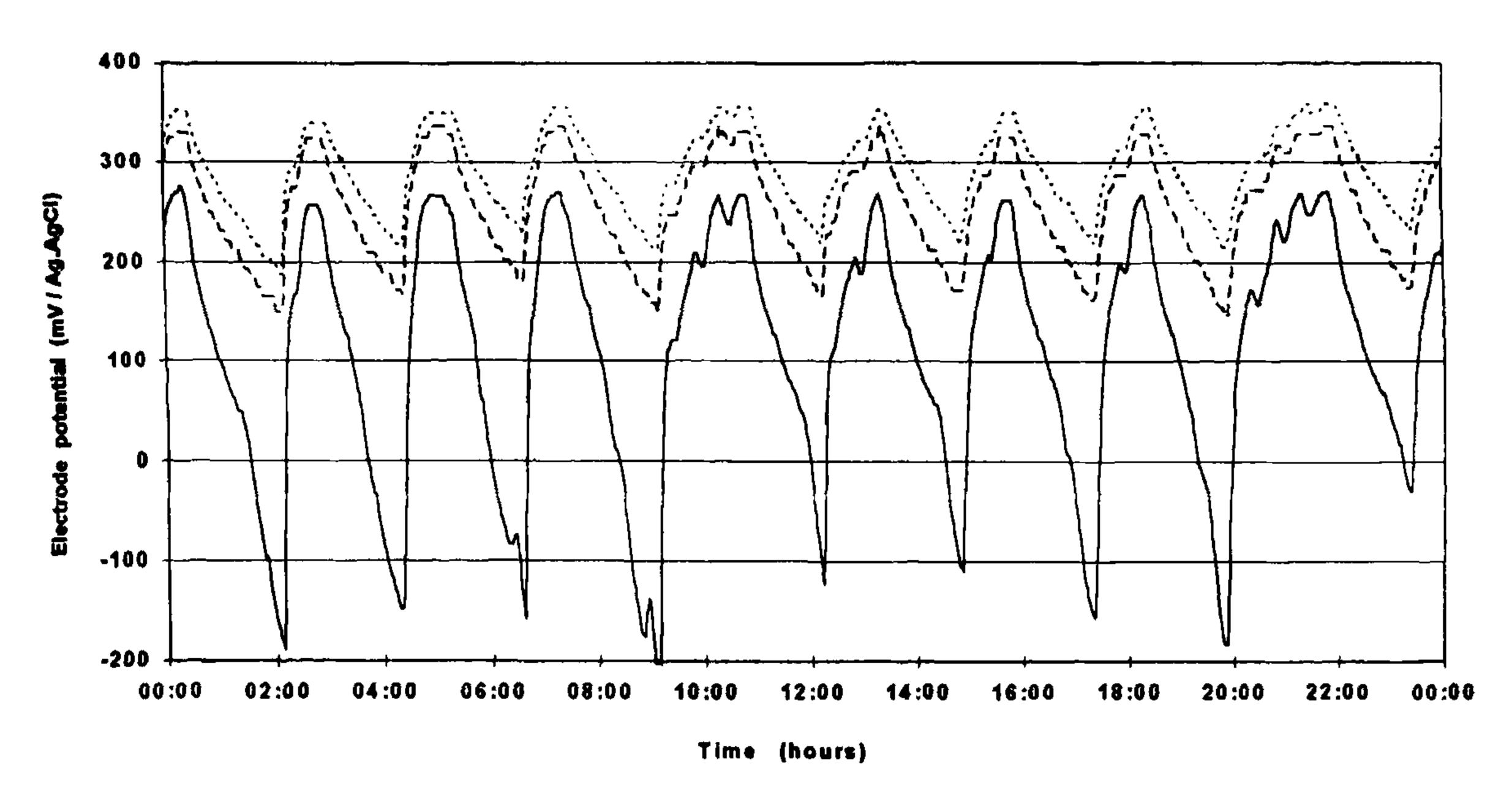
Figure 4. Comparative evolution of the potentials taken by (-) polished electrodes, (---) platinum black electrodes and (...) electrodes coated with platinum black and a Nafion film in sequentially aerated activated sludge.
