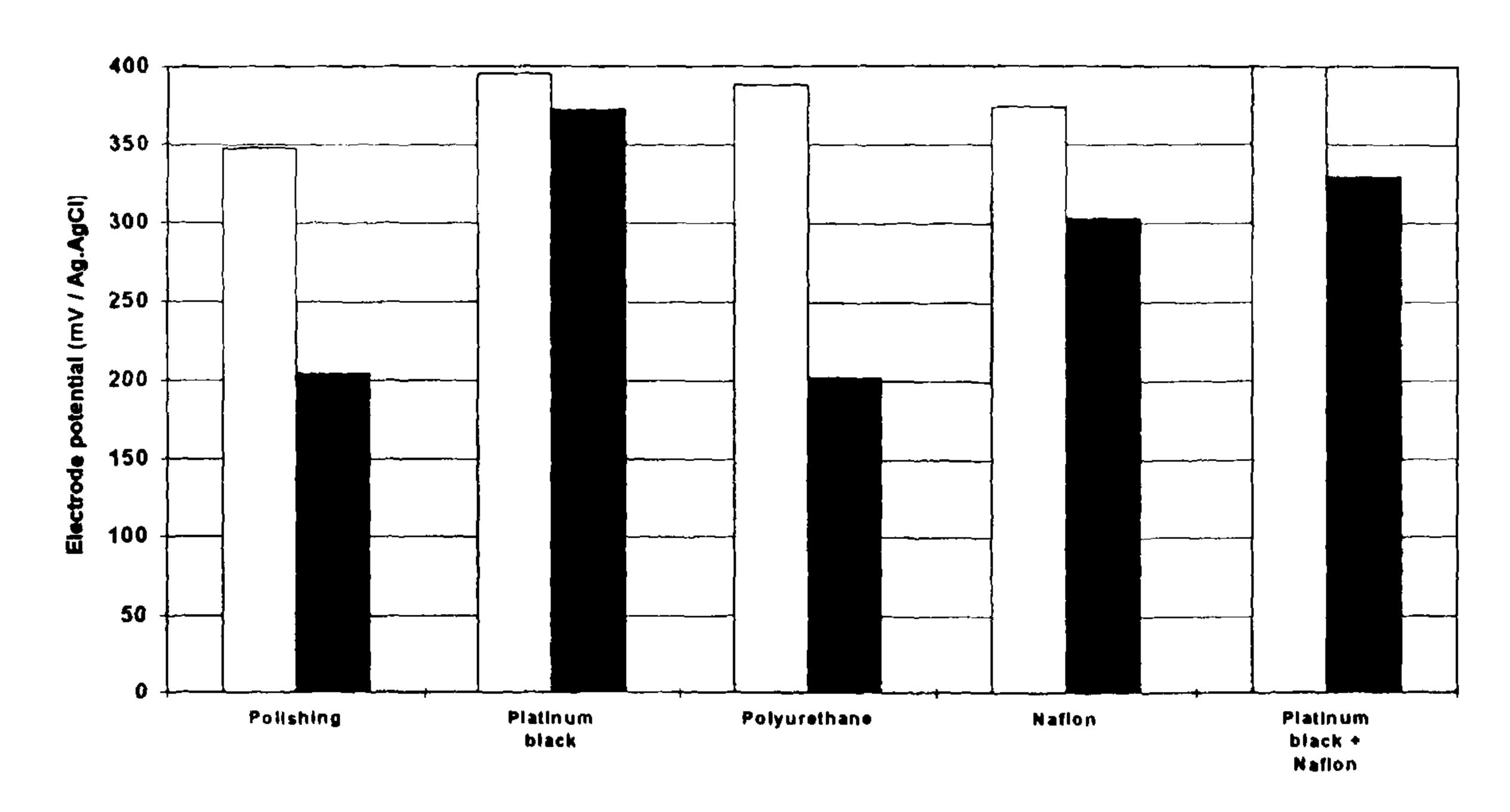
Figure 3. Zero-current potentials of modified electrodes in the PBS reference solution either  $\square$  before or  $\blacksquare$  after a 24 h immersion into anaerobic sludge.
