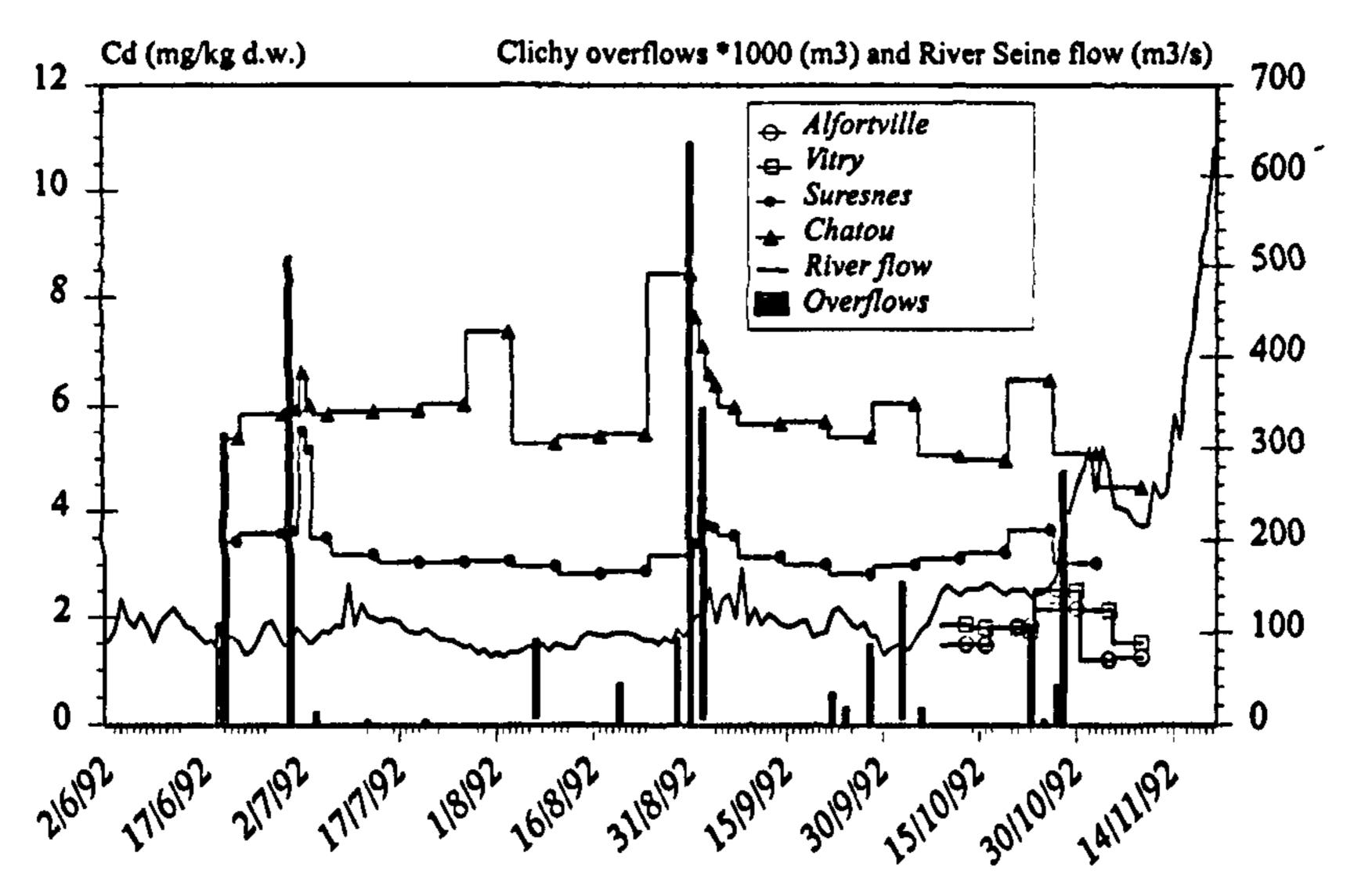
Figure 3. Cadmium concentration variations in river Seine SS from up- to downstream from Paris during summer 1992 (see Fig. 1 for site location).
