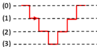
Fig. 1. An iteration procedure of the V-cycle. The grid levels are noted (0) to (3). The red line represents the path that the multigrid algorithm traverses. The dotted lines represent the grid with different spacing.
