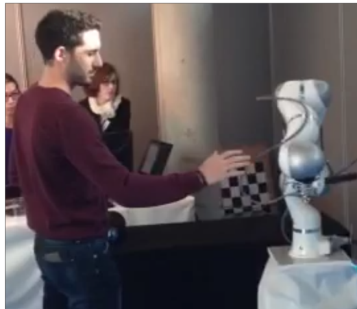
Fig. 1. View of a user sharing its workspace with the KUKA LWR manipulator. The kinetic energy of the system is modulated as a function of the distance between the human operator and the end-effector of the robot in order to best perform the task of the robot while ensuring safety.
