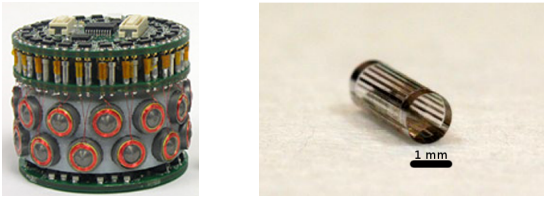
Fig. 1: Claytronics catom prototypes (left one with magnetic actuation, right one with electro-static actuation)
