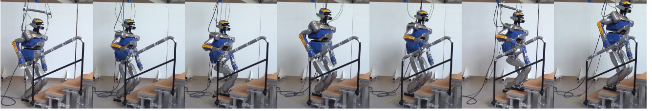
Fig. 3. Set of contact stances realized by the humanoid robot HRP-2 using the method proposed in this paper. The experiment has been realized 5 times in a row without any failure. The companion video shows the realization of the experiment.
