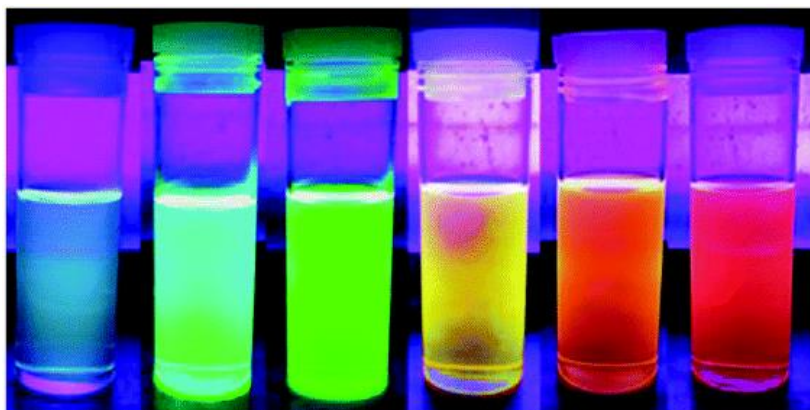
Figure 2 : Photographs of highly luminescent CdSe NCs of various sizes synthesized from cadmium deoxycholate precursor through the continuous mode in supercritical hexane (at P = 10 MPa; 250 °C < T < 310 °C) showing emissions from blue to red regions of the visible spectrum (using UV-lamp at an excitation wavelength of 365 nm).
