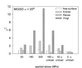
Figure 9 Comparison of the values of  $\chi^2$  obtained from analysis of the MGIXD measurements performed during uniaxial loading and unloading of the austenitic sample. The results for the four grain interaction models are shown.
