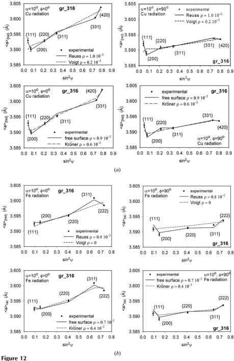
The  $\langle a(\phi,\psi)\rangle_{[hkl]}$  lattice parameters fitted to the experimental points for the AISI316L sample using equation (10) and different types of XSF models. (a) Cu  $K\alpha$  radiation and (b) Fe  $K\alpha$  radiation were used, and the plots for  $\phi = 0^{\circ}$  and for  $\phi = 90^{\circ}$  are shown. The results of the fitting are listed in Table 3; the uncertainty of the peak position is equal to  $\delta(2\theta) = 0.01^{\circ}$ .
