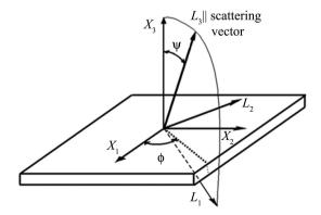
Figure 1 Orientation of the scattering vector with respect to sample frame  $\mathbf{X}$ . The  $\psi$  and  $\phi$  angles define the orientation of the  $\mathbf{L}$  coordinate system (where the  $L_3$  axis is parallel to the scattering vector and the  $L_2$  axis lies in the plane of the sample surface).
