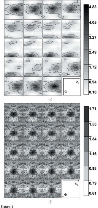
ODFs determined for (a) austenitic stainless steel and (b) polished tungsten. Sections through the basic range  $0 \le \varphi_1$ ,  $\Phi$ ,  $\varphi_2 \le 90^\circ$  of Euler space (Bunge, 1982) with a step of  $5^\circ$  along the  $\varphi_1$  axis for austenitic steel (a) and along the  $\varphi_2$  axis for tungsten (b) are presented.
