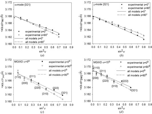
Figure 11 Experimental points and theoretical  $\langle a(\phi, \psi) \rangle_{\{hkl\}}$  versus  $\sin^2 \psi$  plots for a polished tungsten sample. Measurements presented for the standard  $\omega$  geometry (a), the standard  $\chi$  geometry (b), and the MGIXD method with incident angles  $\alpha = 5^{\circ}$  (c) and  $\alpha = 15^{\circ}$  (d) [uncertainty of peak position  $\delta(2\theta) = 0.01^{\circ}$  was assumed].
