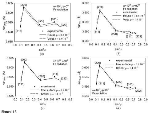
The  $\langle a(\phi,\psi)\rangle_{[hkl]}$  lattice parameters fitted to the experimental points for the polished AISI316L sample (Fe  $K\alpha$  radiation and  $\alpha=10^\circ$ ) using equation (10) and different types of XSF models. Plots for (a), (c)  $\phi=0^\circ$  and for (b), (d)  $\phi=90^\circ$  are shown. The results of the fitting are listed in Table 5; the uncertainty of the peak position is  $\delta(2\theta)=0.01^\circ$ .
