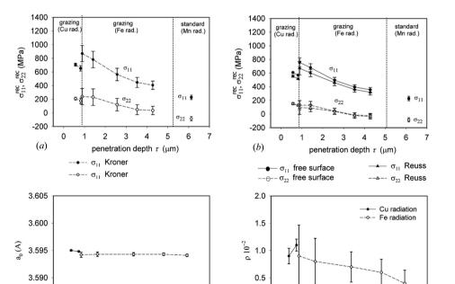
Figure 13 Stress ( $\sigma_{11}^{\rm res}$  and  $\sigma_{22}^{\rm res}$ ), lattice parameter ( $a_0$ ) and the probability of finding stacking faults ( $\rho$ ) plotted *versus* penetration depth  $\tau$  for the ground sample AISI316L. The free-surface model was used to calculate the XSFs. For comparison, the values of stress obtained with the (a) Kröner and (b) Reuss models are shown.
