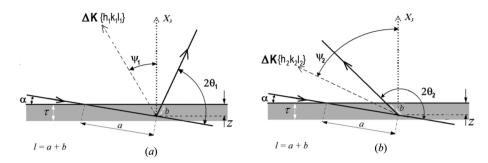
Figure 2 Geometry of the MGIXD method. The incidence angle  $\alpha$  is fixed during measurement, while the orientation of the scattering vector  $\Delta \mathbf{K}_{\{hkl\}}$  is characterized by the angle  $\psi_{\{hkl\}}$ . The depth under the surface and penetration depth are denoted by z and  $\tau$ , respectively.
