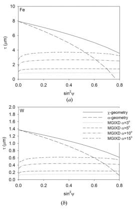
**Figure 3** Penetration depth as a function of  $\sin^2 \psi$  calculated from equations (1), (2) and (4) for (a) austenitic steel ( $\mu = 554 \text{ cm}^{-1}$ , Fe  $K\alpha_1$  radiation) and (b) polished tungsten ( $\mu = 3311 \text{ cm}^{-1}$ , Cu  $K\alpha_1$  radiation). In the standard geometry, the 311 ( $2\theta = 123.5^{\circ}$ ) and 321 ( $2\theta = 131.3^{\circ}$ ) reflections were used for austenitic steel and tungsten, respectively.
