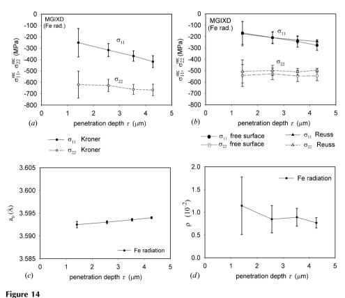
Stress ( $\sigma_{11}^{\text{res}}$  and  $\sigma_{22}^{\text{res}}$ ), lattice parameter ( $a_0$ ) and the probability of finding stacking faults ( $\rho$ ) determined from equation (10), plotted *versus* penetration depth  $\tau$  for the polished AISI316L sample. The free-surface model was used to calculate the XSFs. For comparison, the values of stress obtained with the (a) Kröner and (b) Reuss models are shown.
