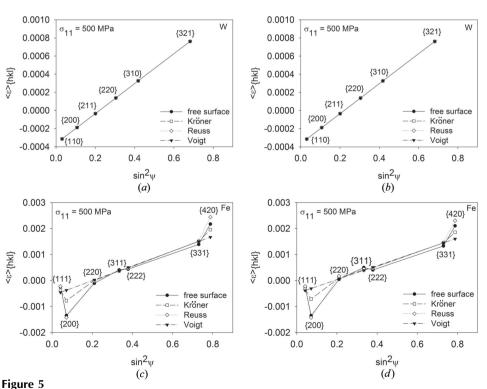
Lattice strains calculated for different hkl reflections used in MGIXD, predicted for uniaxial tensile stress  $\Sigma_{11} = 500$  MPa applied to (a), (b) tungsten and (c), (d) austenitic steel. The XSFs were calculated using the single-crystal elastic constants given in Table 1 and assuming (a), (c) random texture or (b), (d) the experimental texture functions presented in Fig. 4 (in the case of cold-rolled austenite,  $\sigma_{11}$  is parallel to TD).
