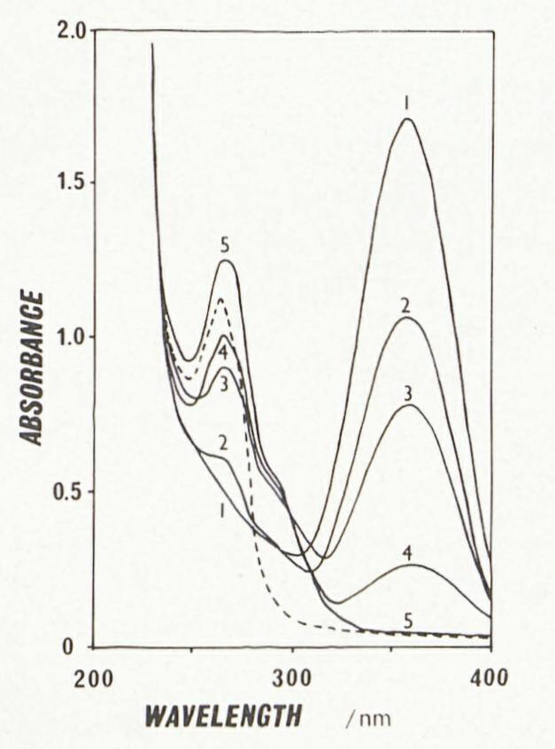
Fig. 2. U.v. spectra of an aqueous  $5 \times 10^{-4} M N_1$ -benzyl-1,4-dihydronicotinamide solution (buffered at pH 8.3) during a macroscale electrolysis at +0.85 V vs. NHE. (1) Initial solution; (2) solution after 0.25,
