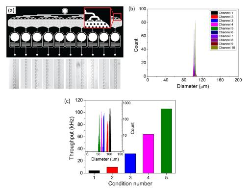
FIG. 2. Droplet production analysis performed with the developed image analysis tool. (a) Example of the recorded highspeed movies from each droplet producer from condition number 1 (channel width:  $100 \ \mu$ m). (b) Histogram of the detected droplet diameter. 18 400 droplets were analyzed from ten droplet producers from condition 1. (c) Measured throughput for each of the five conditions; inset: histogram of droplet diameter for each condition.
