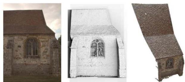
Figure 2: The multi-stereo image matching method: the master image (left), the matching result in the last pyramidal step (center) and the generated colored point cloud (right)
