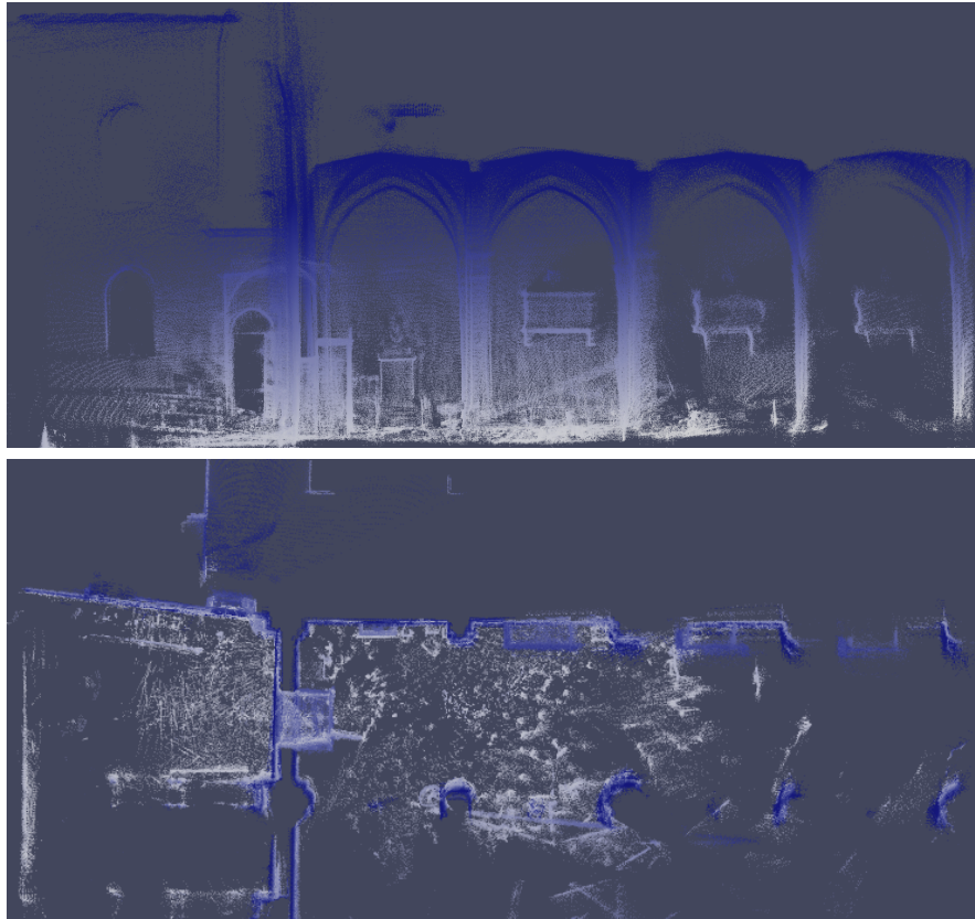
Figure 3.5: Reconstruction of the Chiesa di San Francesco d'Assisi with the color following elevation. Top: Side view of the reconstruction. Bottom: Top view of the church.
