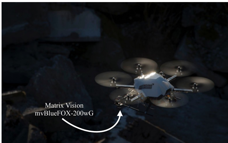
Figure 3.7: Photograph of one of the three AscTec Fireflies used to map the environment in collaboration with the NiftiBot.
