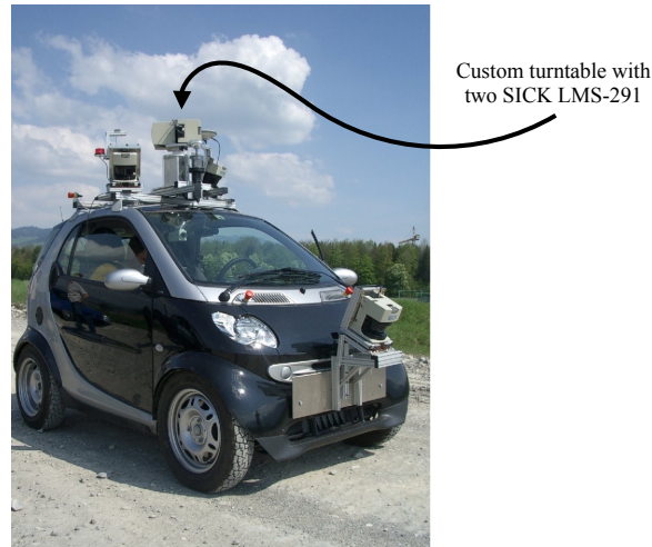
Figure 3.15: The autonomous car, named SmartTer, with its suite of five SICK LMS-291 laser rangefinders. Larger wheels were installed to allow off-road driving.
