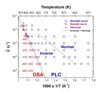
Fig. 4—Map of plastic deformation mechanisms in the temperaturestrain rate plane. PLC denotes the domain in which serrated flow is observed (with either normal or inverse behavior of  $\varepsilon_c$ —see text), and DSA refers to the domain where no serration was observed. Italic numbers close to the open square marks represent the brittle intergranular area proportion on the rupture surface for corresponding tensile test (see text).
