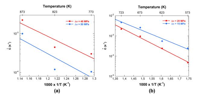
Fig. 10—Plots of strain rate and temperature couples producing given magnitudes of 5 pct plastic deformation stress drops for (a) inverse and (b) normal behavior of  $\varepsilon_c$ .
