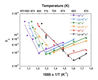
Fig. 5—Variation of the critical strain  $\varepsilon_c$  for the onset of serrations with temperature for given strain rates. The straight lines show normal domain, while the dot lines show inverse domain.
