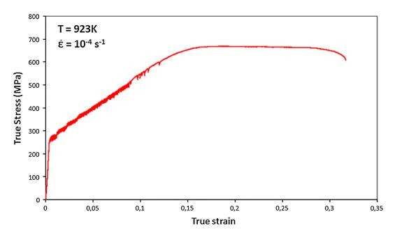
Fig. 11—True stress-true strain curve of a model alloy 718-like without Nb exhibiting PLC effect for testing conditions 923 K (650 °C) to  $10^{-4}$  s<sup>-1</sup>.
