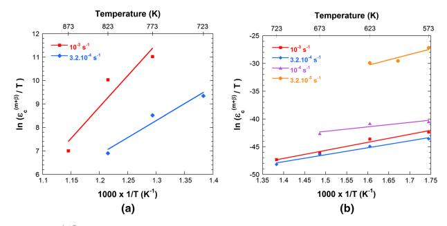
Fig. 7—Plots of  $\log(\varepsilon_c^{(m+\beta)}/T)$  vs 1/T for (a) inverse and (b) normal behavior of  $\varepsilon_c$ .
