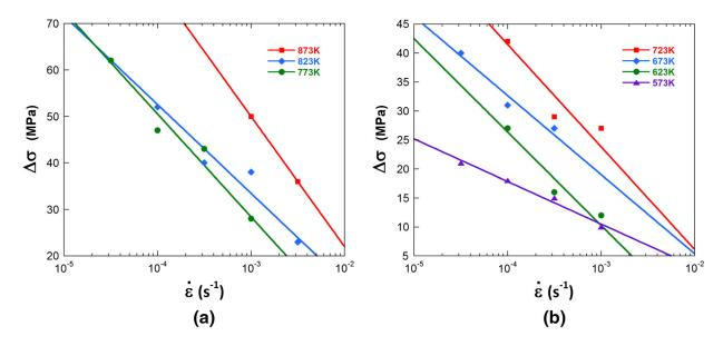
Fig. 9—Variation of the magnitude of stress drops at 5 pct plastic deformation as a function of strain rate for given temperatures (a) for inverse and (b) for normal behavior of  $\varepsilon_c$ .
