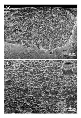
Fig. 3—Rupture surface of a tensile specimen of alloy 718 tested at 873 K (600 °C) in air: (*a*) in the DSA domain- $(3.2 \times 10^{-4} \text{ s}^{-1})$ , and (*b*) in the PLC domain  $(10^{-3} \text{ s}^{-1})$  showing, respectively, the partially intergranular brittle cracking and fully transgranular ductile features.
