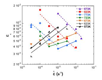
Fig. 6—Variation of the critical strain  $\varepsilon_c$  for the onset of serrations with strain rate for given temperatures. The straight lines show normal domain, while the dot lines show inverse domain.
