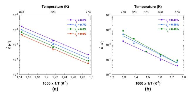
Fig. 8—Plots of strain rate and temperature producing given critical strains  $\varepsilon_c$  for (a) inverse and (b) normal behavior of  $\varepsilon_c$ .
