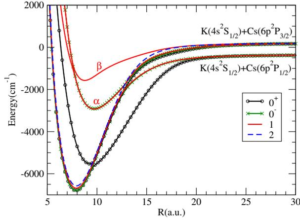
FIG. 2: Hund's case  $c$  potential energy curves of excited molecular states correlating to the dissociation limits  $K(4^2S_{1/2})+Cs(6^2P_{1/2,3/2})$ . The  $\alpha$  and  $\beta$  indexes label the two  $\Omega = 1$  states correlated to the upper dissociation limit.
