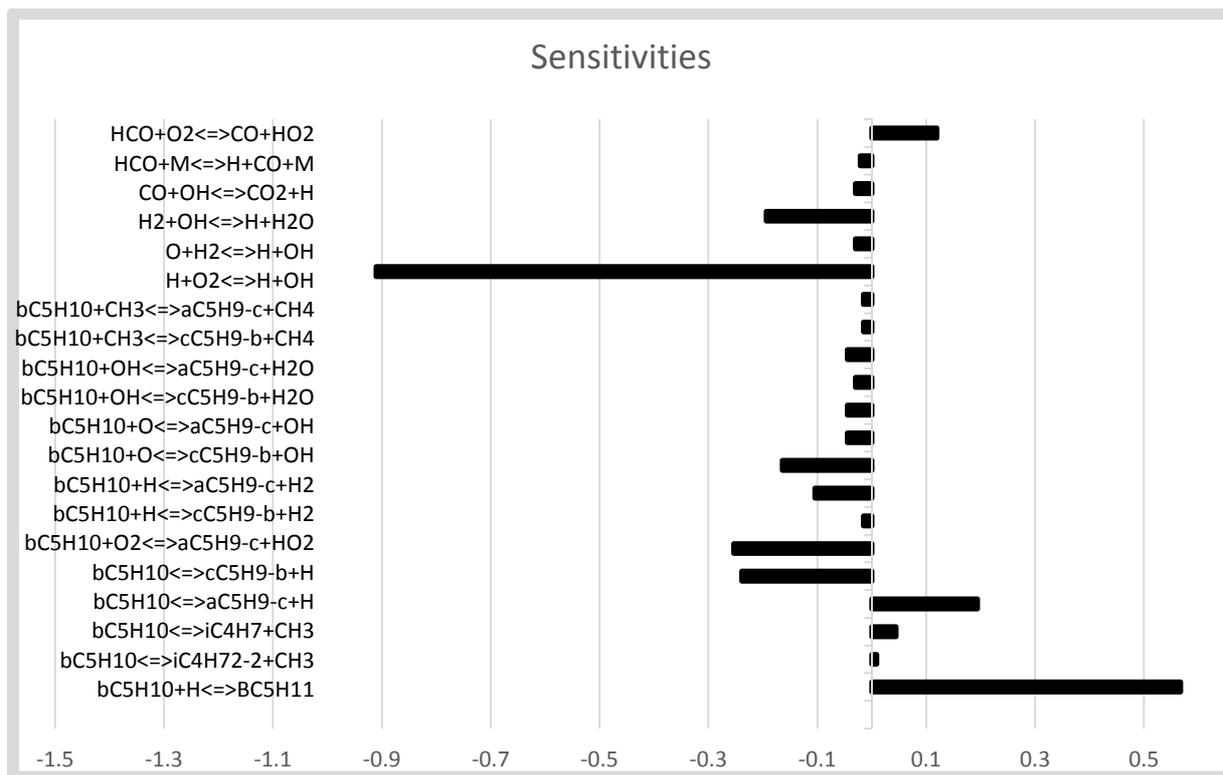
Figure 11: Sensitivity analysis of major reactions in ignition of stoichiometric 2M2B/O<sub>2</sub>/Ar mixture, 0.01 mole fraction fuel, at 11.3 atm pressure and 1500 K, with each rate increased by a factor of 5.
