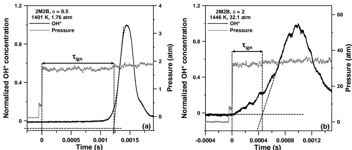
Figure 1: Examples of typical pressure and OH\* profiles and method of determination of the ignition delay time. (a) typical result for most conditions and (b) typical result for  $\phi = 2.0$  above 1.6 atm.
