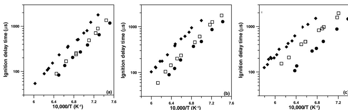
Figure 3: Effect of the pressure on the ignition delay time of 2-methyl-2-butene in 99% Ar at  $\phi =$  (a) 0.5, (b) 1.0, and (c) 2.0.  $\blacklozenge$  show results at about 1.7 atm,  $\square$  show results at about 11 atm, and the  $\bullet$  show results at about 31 atm.
