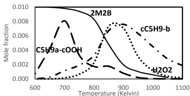
Figure 12: Computed mole fractions of fuel 2M2B and selected representative metastable intermediates in JSR simulations at 1.06 bar pressure and residence time of 1.5 s. The mole fractions of  $C_5H_9a-cOOH$  have been multiplied by 107, the mole fractions of  $cC_5H_9-b$  have been multiplied by 3000, and the mole fractions of  $H_2O_2$  have been multiplied by 20, to permit comparisons in behavior.
